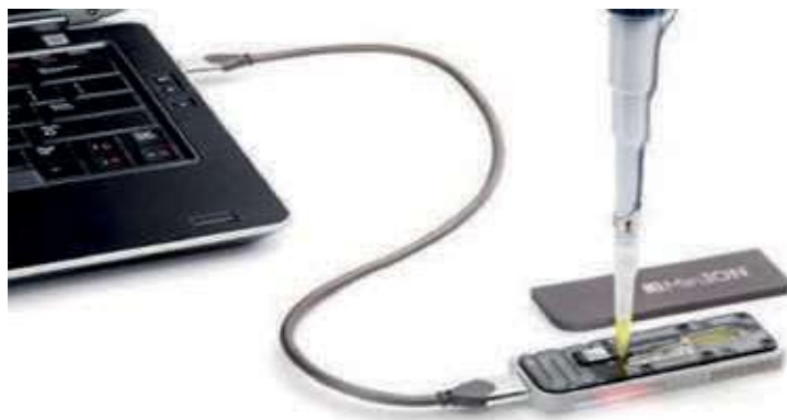
Figure 4 - Third-generation sequencing. The figure illustrates the compact spatial requirements of the nanopore technology, which encompasses both the chip and the laptop computer. These requirements are sufficient to facilitate the execution of sequencing procedures in real-time and in situ analysis.
