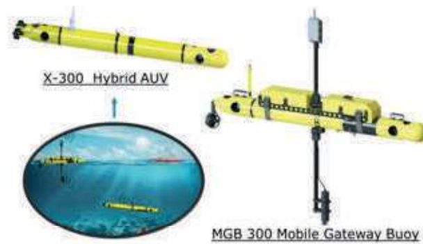
Figure 2 - Representation of the vignette illustrating multi-vehicle cooperation, highlighting the interaction between an underwater autonomous vehicle, a surface vehicle, and the support naval unit.
