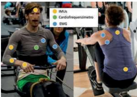
Figure 2 - Positioning of the sensor wearable for the sports practice of para-rowing.
