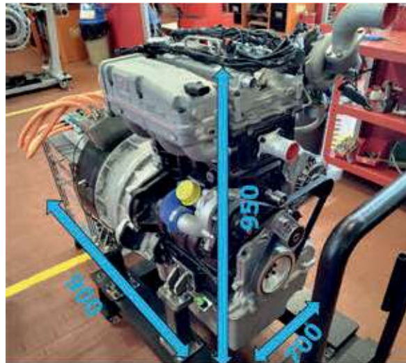
Figure 4 - Overall dimensions of the 2CHDP hybrid group.
