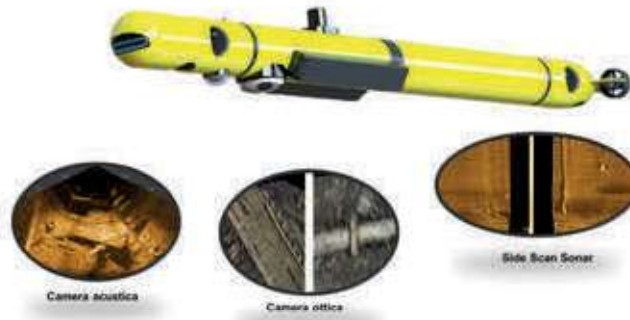
Figure 1 - Render of the autonomous vehicle X300 designed for the PNRM PACMAN. Specifically, the sensors equipped on the vehicle for the detection, classification, and recognition of potential underwater threats are highlighted.
