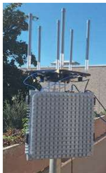
Figure 6 - The interferometric system (5 antenna version). The developed system can be configured with any number of antennas, however arranged.
