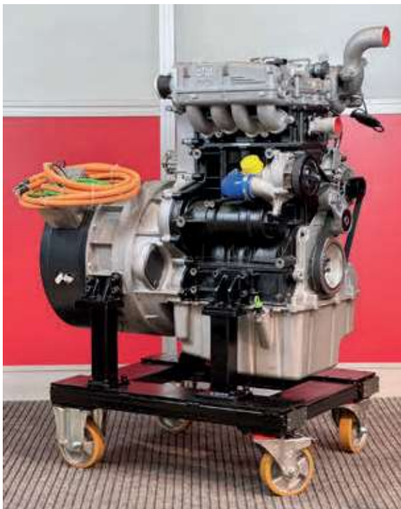
Figure 7 - Assembled engine ready for test bench.
