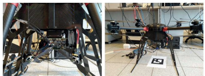
Figure 4: Intelligent Payload deployed on-board of a multi-rotor drone
