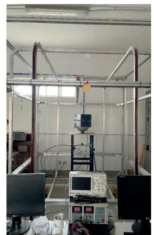
Figure 3 - Attitude test of satellite in Helmholtz chamber
