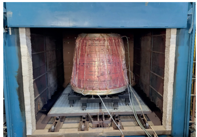
Resin infusion and oven curing
